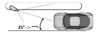
Once the camera is installed, check that the number plate is not too far off-horizontal in such a way as to **exceed 5°** in either direction as this could make it difficult to correctly read the registration.
